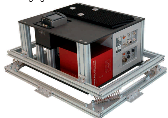
Image showing laser scanner of LiteMapper system with IMU of AEROcontrol and DigiCAM
